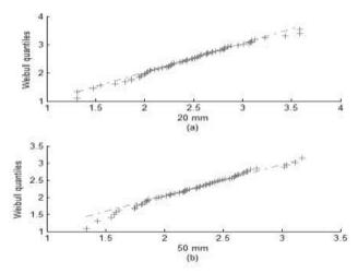
Figure 1. Weibull Q-Q plots of gauge lengths of 20 mm (a) and 50 mm (b) data
